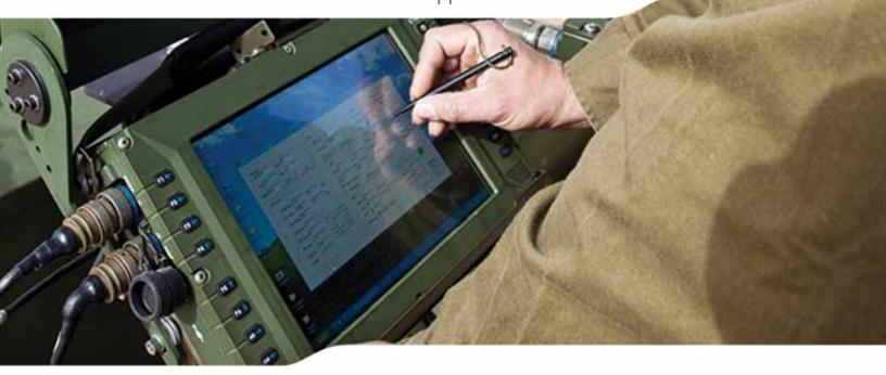
The TACTER®-31D is an indispensible command and control tool for the modern digital battlefield, ensuring complete continuity across vehicle-mounted and dismounted applications. Establishing new performance standards, the ruggedized tablet computer is compliant with MIL-STD-810F and MIL-STD-461E, and features embedded MIL-STD-1275D power conditioning. The light-weight tablet configuration and integrated handle allow the unit to be quickly and easily transported.
